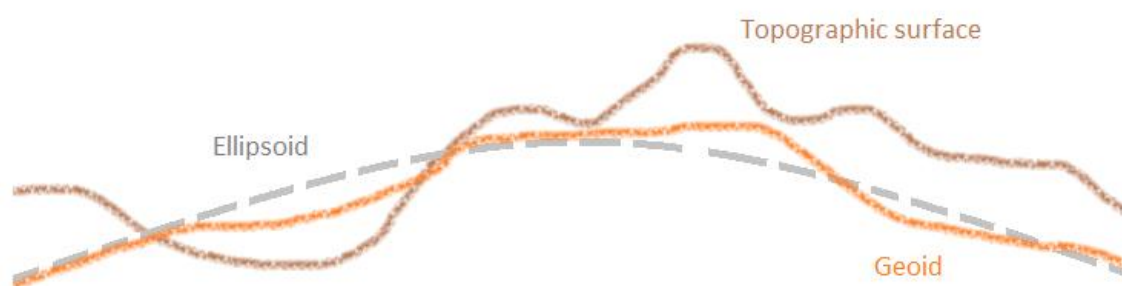
Figure 3. Relationship between geoid, topographic surface and ellipsoid fitting. Image Credit: Peter H. Dana, 1994.
